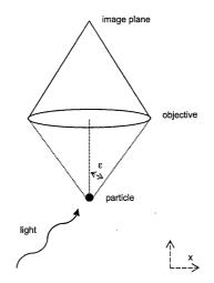
FIGURE 1: Schematized light microscope
